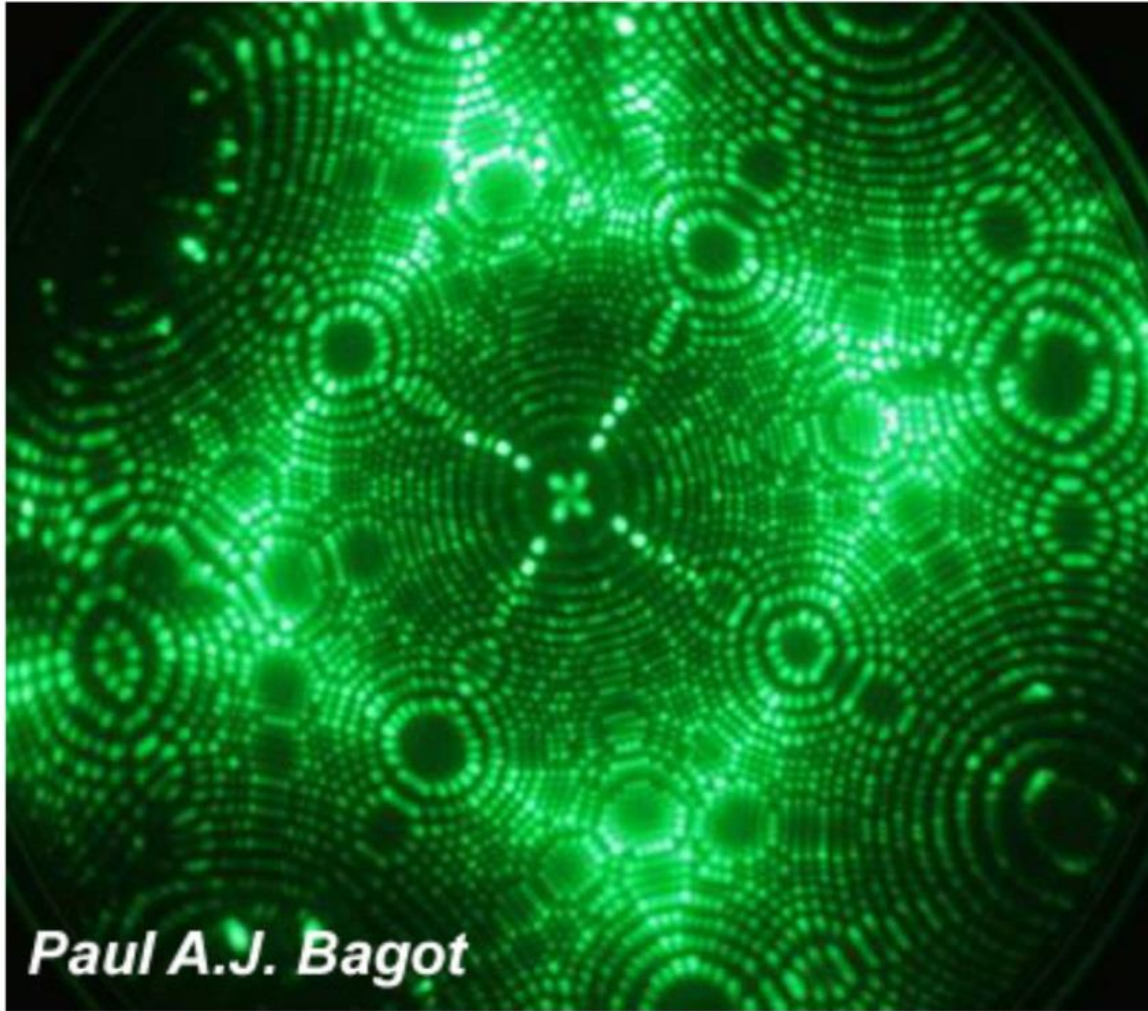
Pt surface imaged using field ion microscopy for catalysis research
